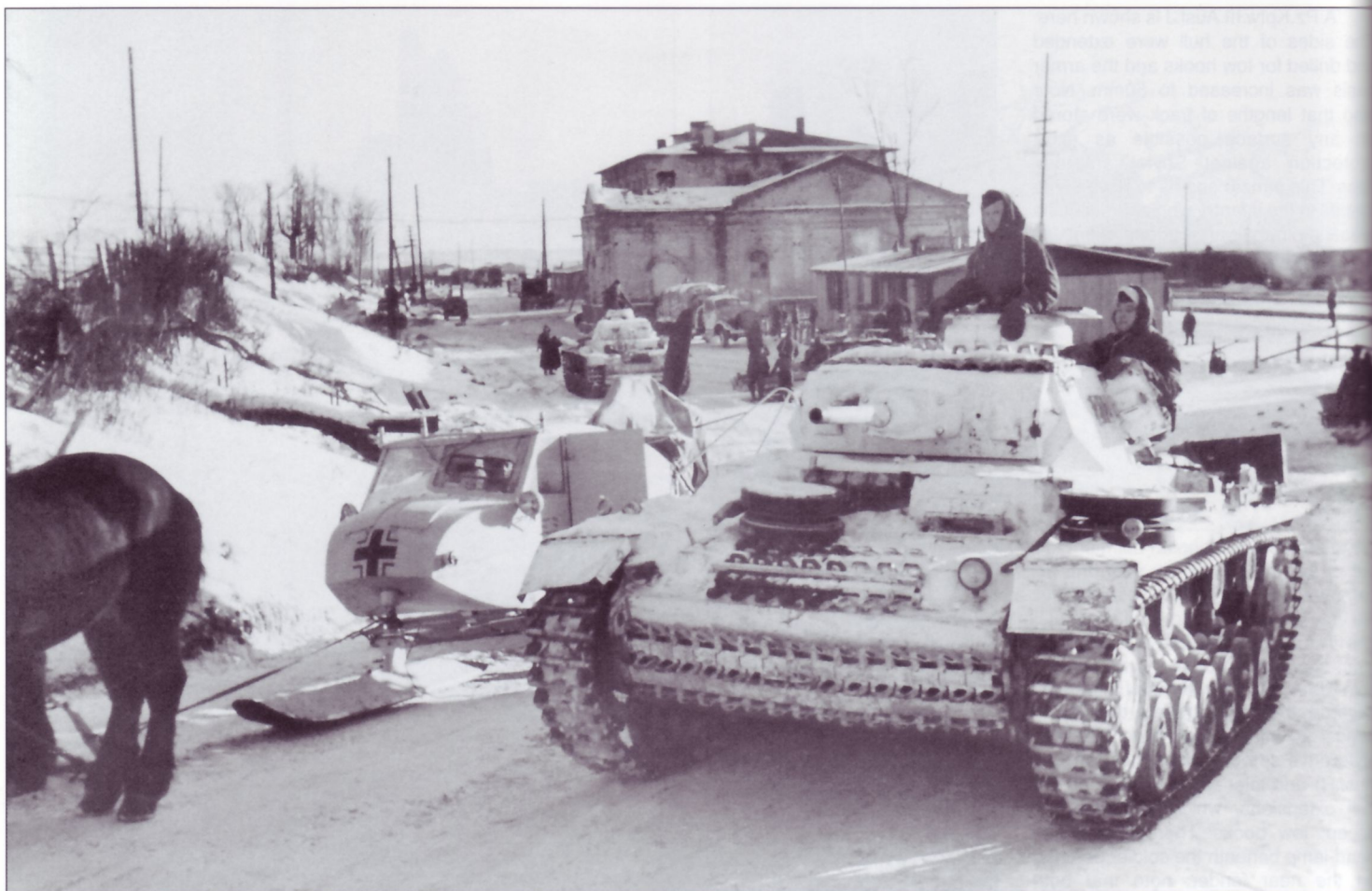
A relatively neatly white-washed Pz.Kpfw.III Ausf.J moves along a road during a winter on the Ostfront. There is a tactical number, in white on an uncamouflaged rectangle on the turret sides, possibly "212". Again, note the new drive sprocket as well as the new idler wheel, and the hull extensions drilled to accept a tow hook. Behind the panzer is a uniquely-Soviet snow vehicle, called an "Aerosan", in this case being towed by a local pony. The captured Aerosan sports a balkenkreuz on the nose of its white-painted body.
