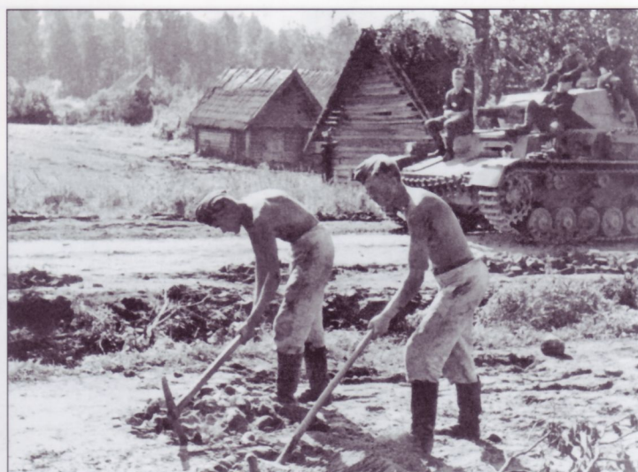
This Pz.kpfw.IV Ausf.C passes a pair of pioniere troops (combat engineers) busily engaged in digging. The panzer is identified as an Ausf.C by the configuration of the view ports on the superstructure front. There is length of spare track fitted to the bow and an improvised jerry can rack on the fender. The turret has been retro-fitted with a storage bin, a very common occurrence.
