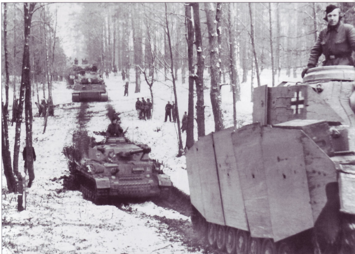
A pair of Pz.Kpfw.IV Ausf.Hs lead Tiger Is of SS-Division "Das Reich" along a forest track, on the Ostfront. The lead panzer is identified as an Ausf.H by the new drive sprocket which could not be fitted to an Ausf.G hull, unless the transmission and final drives were also changed. It has a single-piece lid on the commander's cupola as well as Zimmerit anti-magnetic mine paste, which was applied at the factory to panzers beginning in September of 1943. Note the cut-out portion of the small Schürzen plate just over the drive sprocket. The panzer is finished in the base of dunkelgelb RAL 7028 and has only a white-outlined, black balkenkreuz visible on the turret Schürzen. Other panzers in the column have the divisional insignia left-over from "Operation Zitadelle" (a horizontal bar with a pair of attached vertical bars, in white), which took place the previous July.
