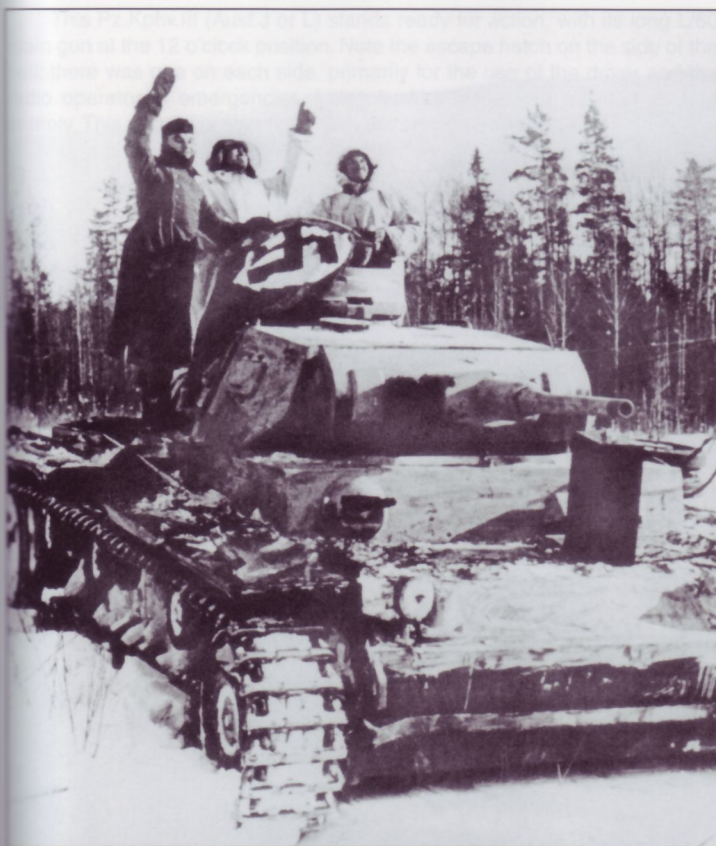
Taking no chances on being attacked by friendly aircraft, this crew of a Pz.Kpfw.III Ausf.J gestures and waves their Nazi aerial recognition flag towards the sky. This panzer has a rather worn white-wash applied; note how the area behind the removed track storage on the bow has not been covered in white.
