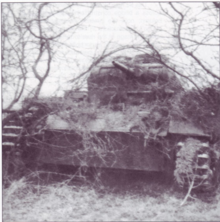
A partially-camouflaged Pz.Kpfw.III Ausf.E stands idle while awaiting the order to continue the assault. While the camouflage is not especially elaborate, it succeeds in breaking up the vehicle's outline and also blends in well with the surrounding trees. This panzer has a Notek head-lamp mounted on the driver's side of the glacis plate, but is otherwise devoid of any other unique or unusual features.
