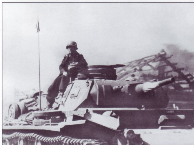
This Pz.Kpfw.III Ausf.J, shows its chassis number, possibly 68435 on the superstructure front, to the left of the driver's pivoting visor. There is also a single-digit tactical number, a white-outlined "7" on the forward side of the turret, and a sprayed outline of a European Bison just behind it, identifying this panzer as belonging to Panzer-Regiment 7, originally of the 10.Panzer-Division. It flies a pennant from its rod antenna. Unusually, the crewman perched on the turret wears his steel helmet.
