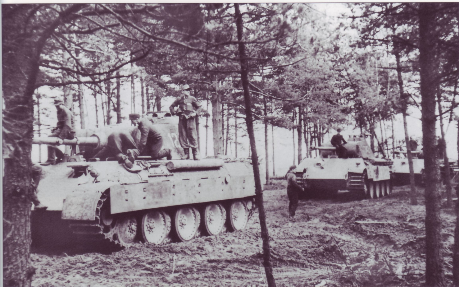
This column of Panthers is led by an Ausf.A (note the cast cupola), which has the full front mud-flap extensions. The 7.5cm KwK42 L/70 gun is resting in the travel crutch. It would appear that the second Panther is an Ausf.G, since there is no view-flap on the upper glacis plate, although at this distance it's hard to say. The Ausf.A has parts of a tactical number, in white, visible on the side of the turret, but is otherwise unremarkable in appearance.
