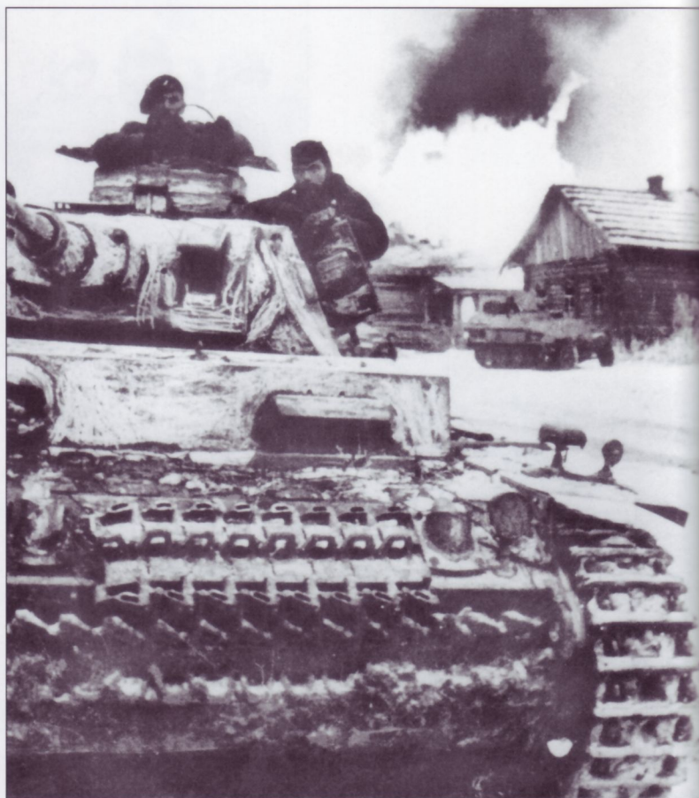
A relatively neatly white-washed Pz.Kpfw.III Ausf.J moves along a road during a winter on the Ostfront. There is a tactical number, in white on an uncamouflaged rectangle on the turret sides, possibly "212". Again, note the new drive sprocket as well as the new idler wheel, and the hull extensions drilled to accept a tow hook. Behind the panzer is a uniquely-Soviet snow vehicle, called an "Aerosan", in this case being towed by a local pony. The captured Aerosan sports a balkenkreuz on the nose of its white-painted body.
