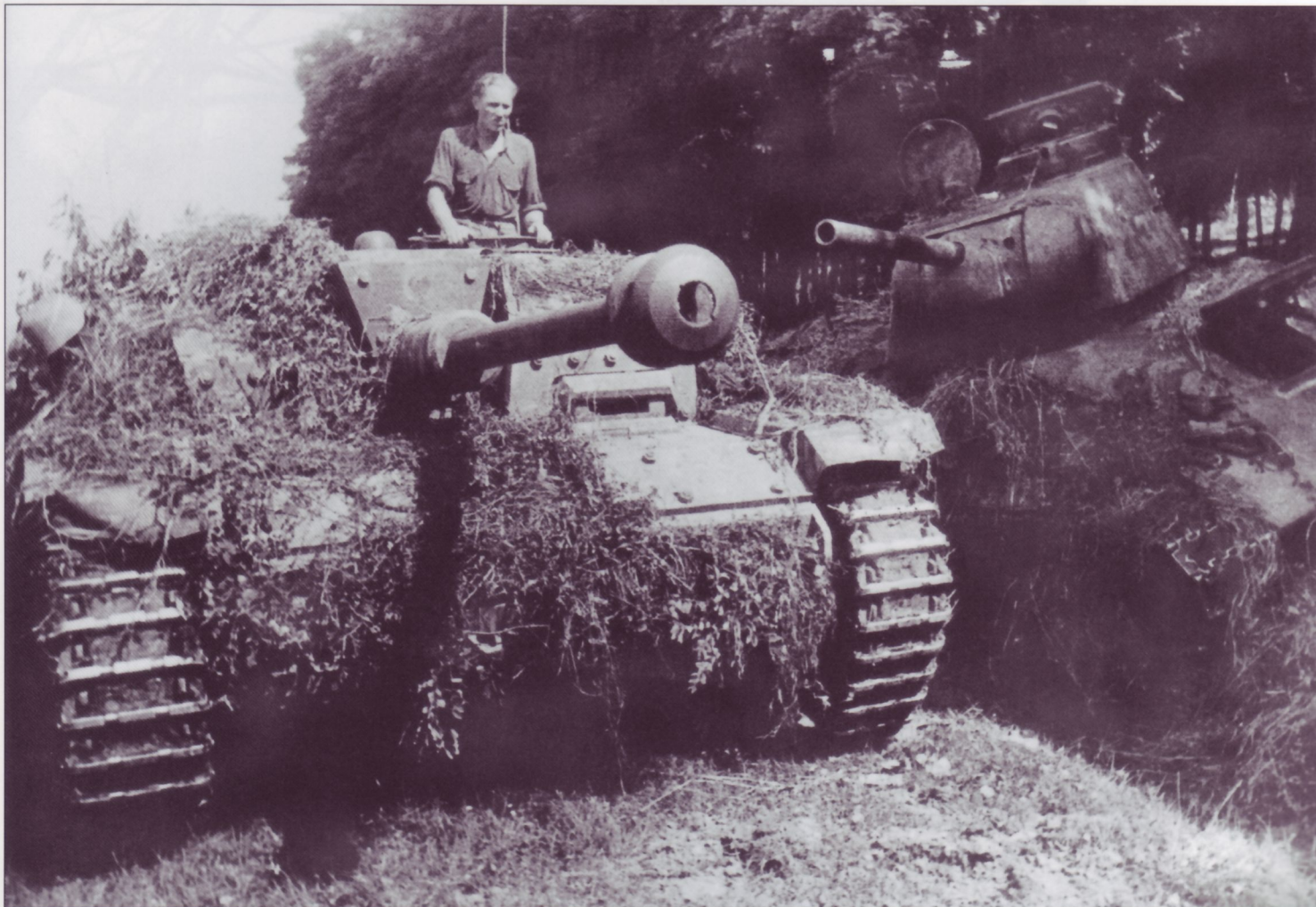
A well-camouflaged StuG.III Ausf.G passes a knocked-out Soviet T-34 Model 1943 with a commander's cupola and sharp-nose hull front (characteristic of tanks produced at Factory 174 during the spring of 1943). The assault gun has bolted-on 30mm appliqué plates on the upper and lower glacis plates as well as the front plate of the driver's compartment. Those plates were originally 50mm, so the vehicle now had 80mm of armor plate on its front. The only stowage of note is the steel helmets, one on the roof, with another on the superstructure side.
