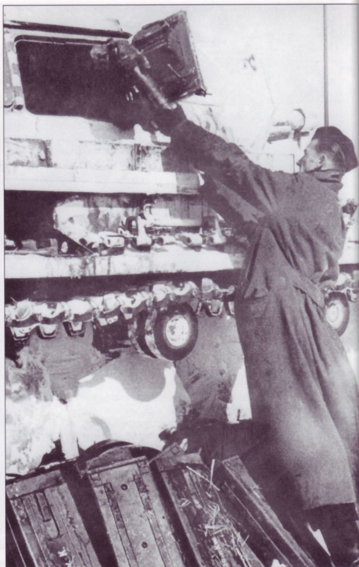
A crewman hands a 5cm round to his comrade in the turret of a Pz.Kpfw.III, probably an Ausf.F. A number of later Ausf.F were produced with the short 5cm KwK38 L/42, while some had this weapon retro-fitted during major overhauls. This panzer has a winter white-wash applied, but is otherwise devoid of any other special items of interest. The crewman wears the M1935 greatcoat over his uniform with his M1934 field cap perched at a jaunty angle on his head. Note the ammunition boxes leaning against the road-wheels at the bottom of the photo.
