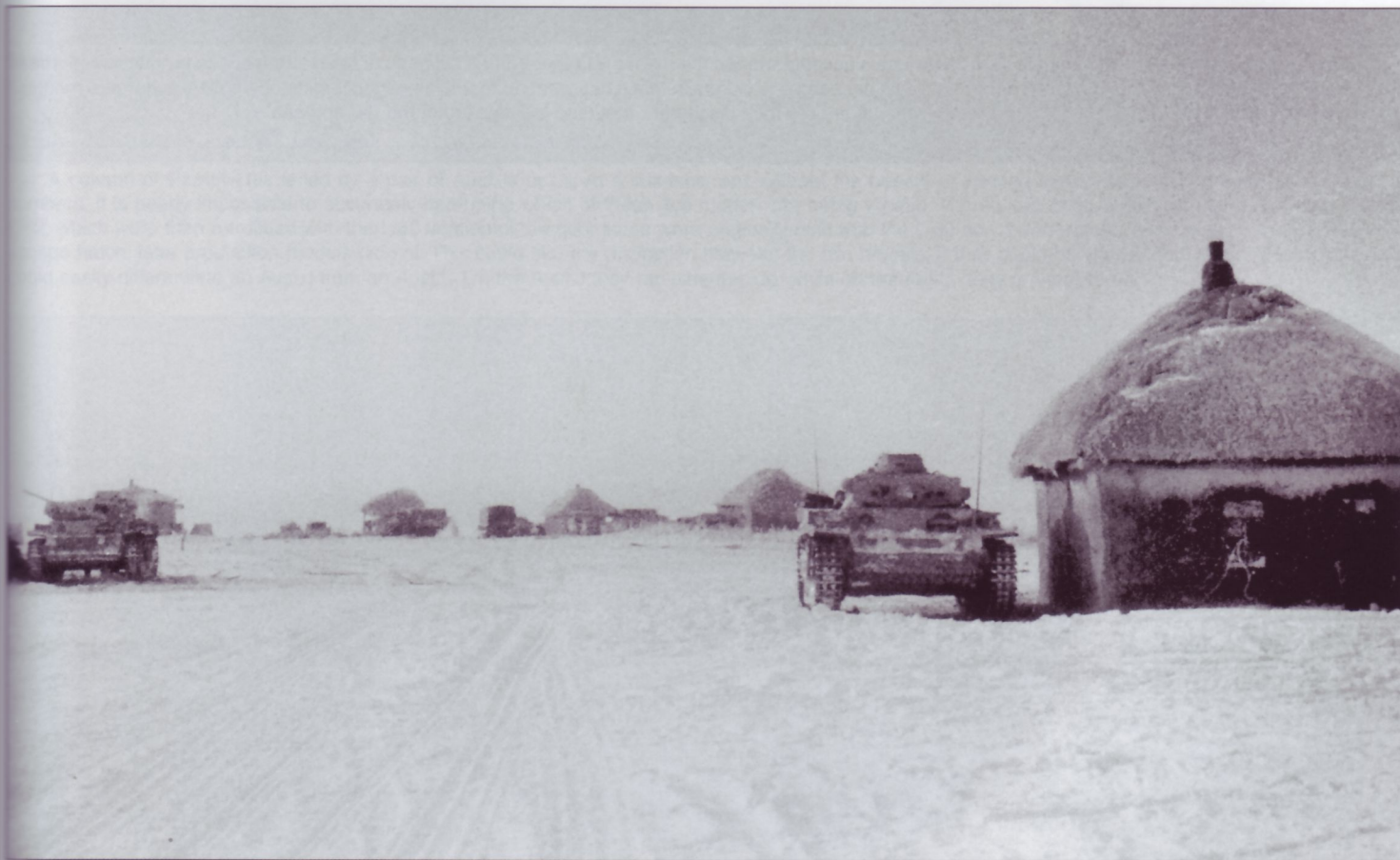
A Befehls-panzer, based on the Pz.Kpfw.III Ausf.J or L sits next to a peasant's home on the open steppes of the Soviet Union. There are two rod antenna masts, one on either side of the panzer, as well as 20mm spaced armor on the mantle and the superstructure front plates. This panzer also seems to be mounting the longer L/60 version of the 5cm KwK39 main gun.
