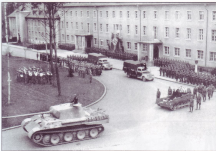
A Panther Ausf.D leads a funeral procession with the deceased's coffin mounted on a stripped-down Pz.Kpfw.I chassis. Note the cupola and its open hatch lid as well as the extended front mud guards. The Panther also has Zimmerit applied; note the bare areas on the forward superstructure sides where standard tool stowage has been removed.
