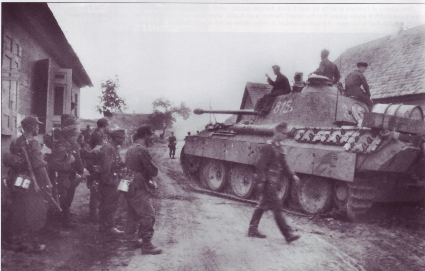
A heavily stowed Panther Ausf.A awaits orders to pull out, under the watchful eyes of a group of infantrymen. Aside from the usual tool, cable and spare track stowage, this panzer also carries a large wood beam, probably for use in extricating itself from ditches. There is also a 200-liter fuel drum on the engine deck (indicating a road march is being contemplated) and a bucket hanging from the triple exhaust pipe on the hull rear. It carries a full set of Schürzen, while the vehicle jack is stored in a later horizontal position. The relatively crudely applied tactical number ("815" in yellow or white) places this panzer in the 8.Kompanie of a Panzer-Regiment's II.Abteilung. The panzer is coated in Zimmerit and finished in a base of dunkelgelb, with patches of a secondary color.
