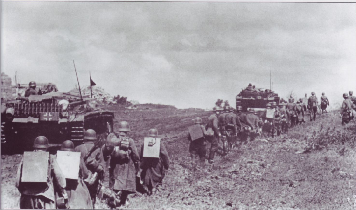
A pair of StuG.IIIs (at this angle, they could be either Ausf.B, C, D or E) pass a section of radio-equipped troops, somewhere on the Ostfront. As the periods of combat lengthened, the supply situation for Germany steadily worsened. Thus, many combat vehicles began carrying large amounts of spares and consumables. The near assault gun typifies this trend by mounting spare tracks on its engine deck, which also act as a framework to keep other loose items in place, such as the buckets towards the left.
