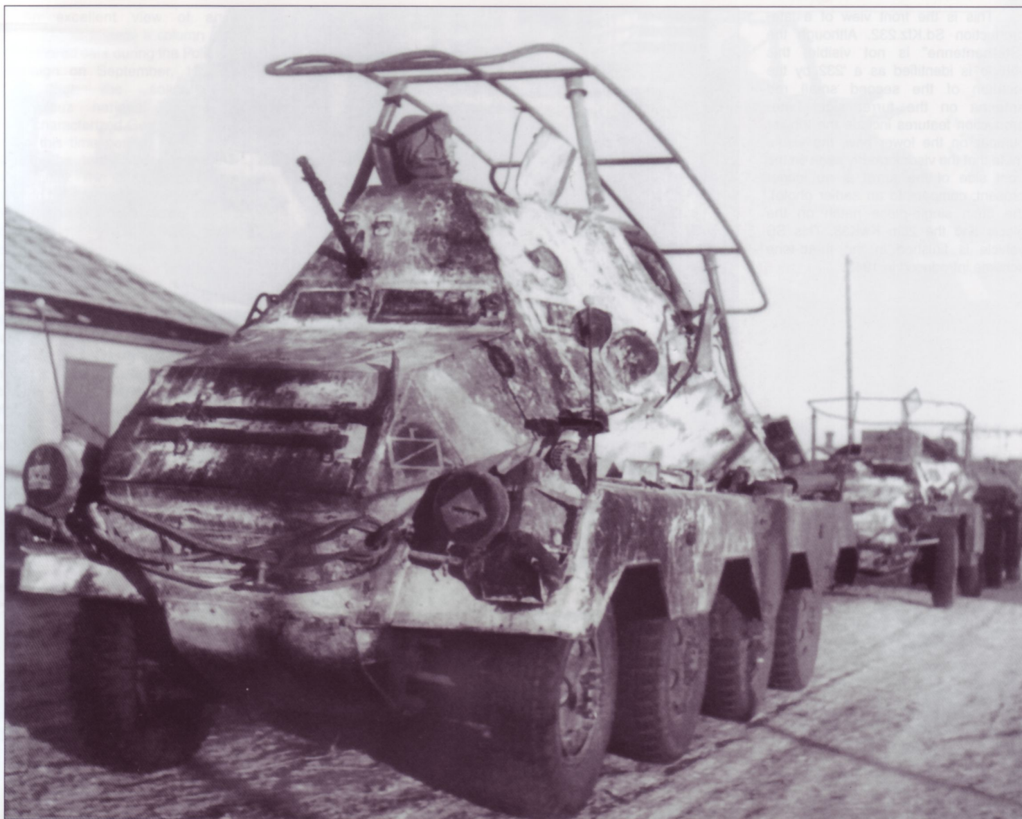
This Sd.Kfz. 263 contains later features, notably the visors, which were of a standardized, cast design that dispensed with the need for rain gutters above them. It is finished in a very worn white-wash over what should be a base of dunkelgrau. The tactical sign signifies a headquarters element from either a motorized infantry battalion or motorcycle reconnaissance battalion. An Sd.Kfz. 223 follows behind.
