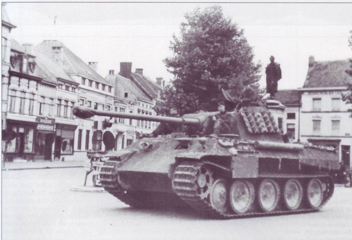
This Panther Ausf.D has an earlier turret with an "MP Stopfen" (machine-pistol port with plug) on the rear plate, to the left of the escape hatch. It is missing the external gun travel crutch, which should be in place over the ventilation fan cover, on the center of the forward edge of the hull roof.
