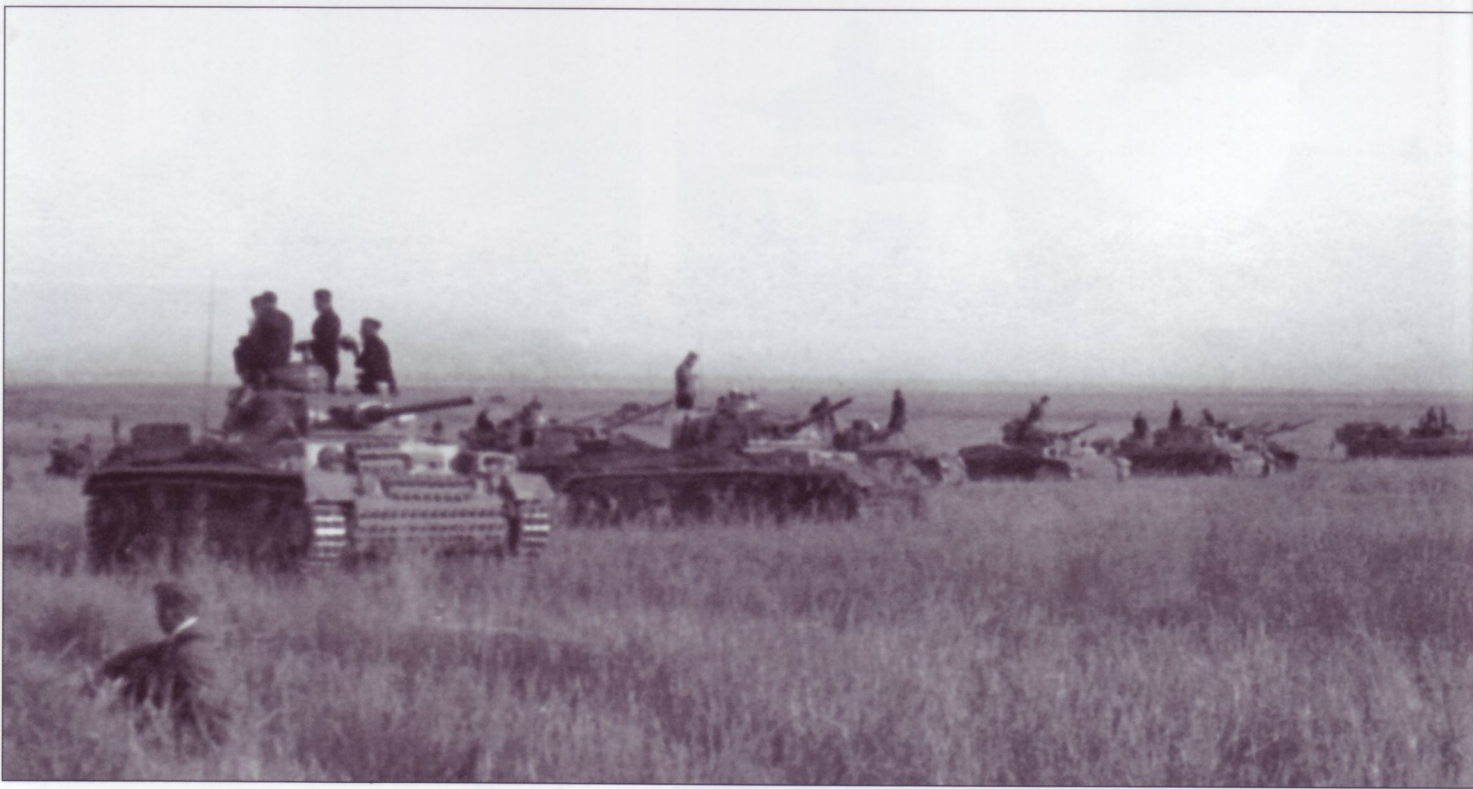
A company-sized detachment of Pz.Kpfw.IIIs (Ausf.J or L) relax on the steppes of the Soviet Union. Some, such as the second panzer from the left have appliqué spaced-armor arrays (although it only has the frame for the array on the mantle), while others do not.
