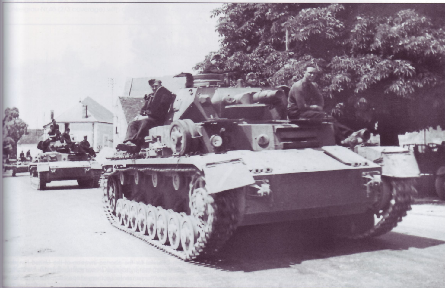
A Pz.Kpfw.IV Ausf.D leads a column of panzers through a town, probably after the French Campaign of 1940; note that the black beret is not worn, it being discarded shortly after the end of the battles in the west. There are no markings visible on this dusty panzer, while the only unique fitting is a frame to store a spare road wheel mounted on the near fender. This view also affords a better look at the radio antenna deflector strapped on to the gun tube.
