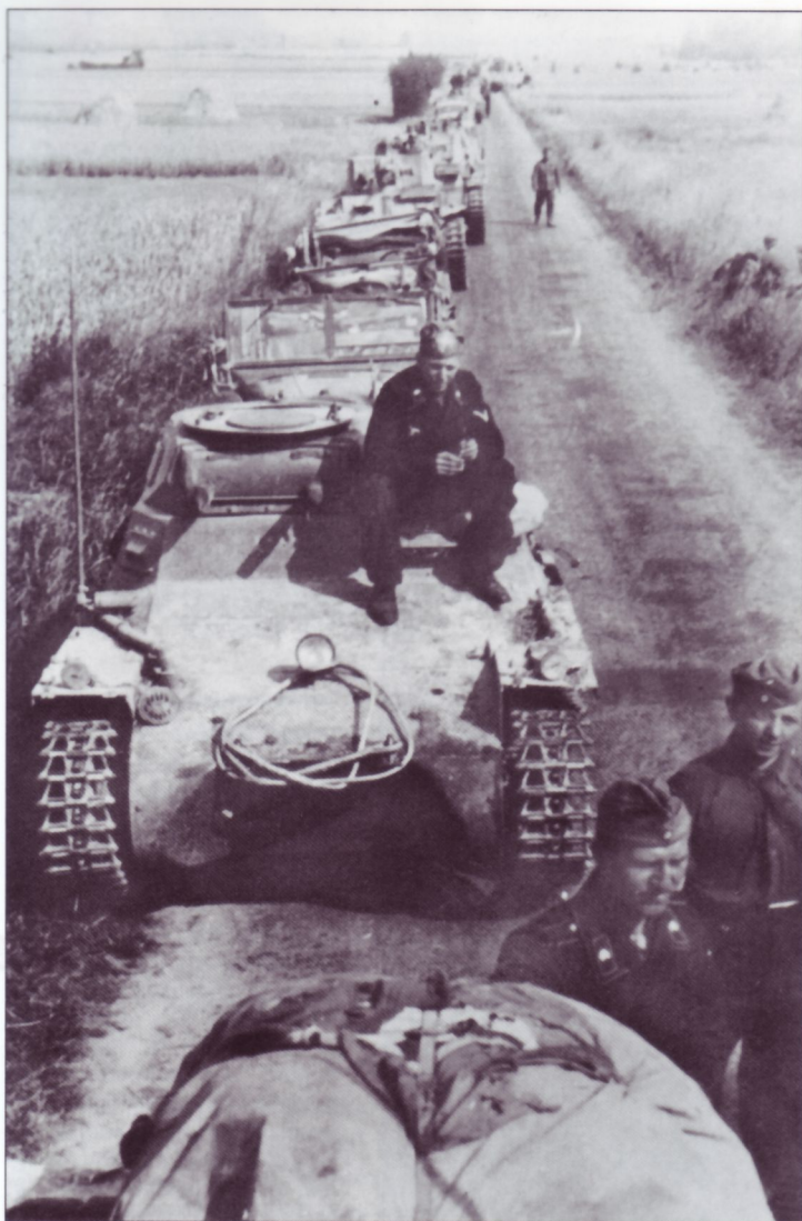
A Pz.Kpfw.I Ausf.B leads a column consisting of wheeled vehicles and Pz.Kpfw.38(t)s, during the French Campaign. From this angle the panzer is identified as an Ausf.B by the lack of a vehicle jack stowed on the right front fender (although some Ausf.Bs did, in fact, have a jack stowed in that position). A close look at the superstructure, next to the radio antenna, as well as the front plate will reveal an inverted "Y" with three dots, which was the divisional insignia of 7.Panzer-Division, which was equipped with the Pz.Kpfw.38(t); this marking is seen on one of those panzers later in this book.
