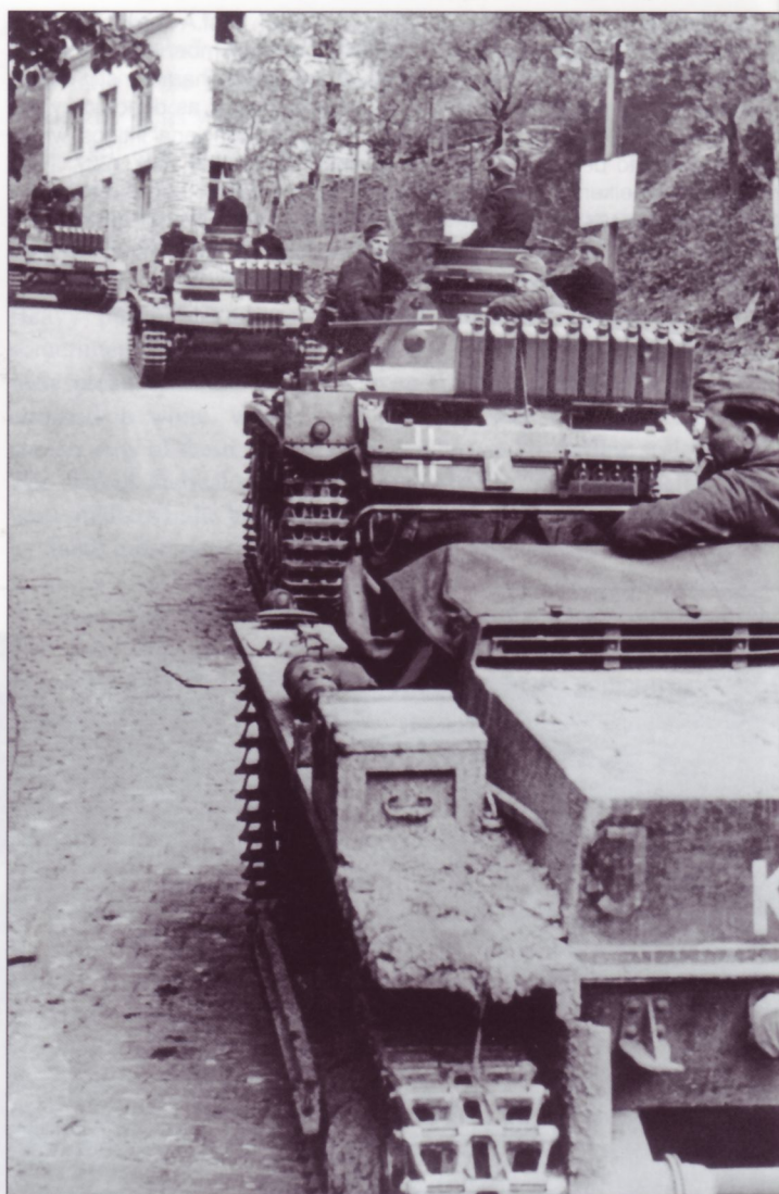
A column of Pz.Kpfw.III (Ausf.D, E or F) leads a Pz.Kpfw.I Ausf. B ohne Aufbau, which has been converted into a vehicle to carry maintenance equipment for the panzer company's repair and recovery sections, by the removal of its superstructure and turret. It was also known as "Instandsetzungskraftwagen I". Note the yellow gothic "I" (which appears to be a "J") that identifies the vehicle's function, on the rear corner of the engine deck, as well as the white "K" of Panzergruppe von Kleist. Note also the small square tactical markings on the rear turret face of the Pz.Kpfw.IIIs and the racks for jerry cans on their rear decks.
