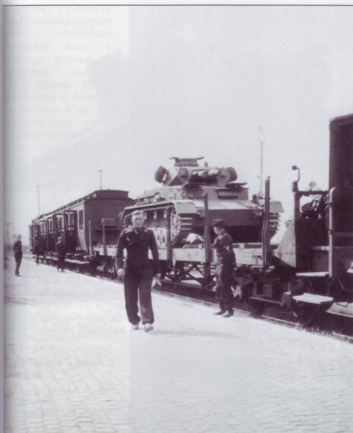
A lone Pz.Kpfw.IV Ausf.C sits on a platform wagon at a rail-head. The panzer is identifiable as an Ausf.C by the arrangement of the view ports on the superstructure front. Note also that the cupola differs from that of the Ausf.A seen in the previous photograph. There are no markings visible, while the crew members wear the black M1934 panzer uniform, along with the characteristic large black beret. Typically, the Germans did not chain tracked vehicles to rail wagons, preferring instead to use wooden blocks and chocks to prevent fore-to-aft and side-to-side movement.
