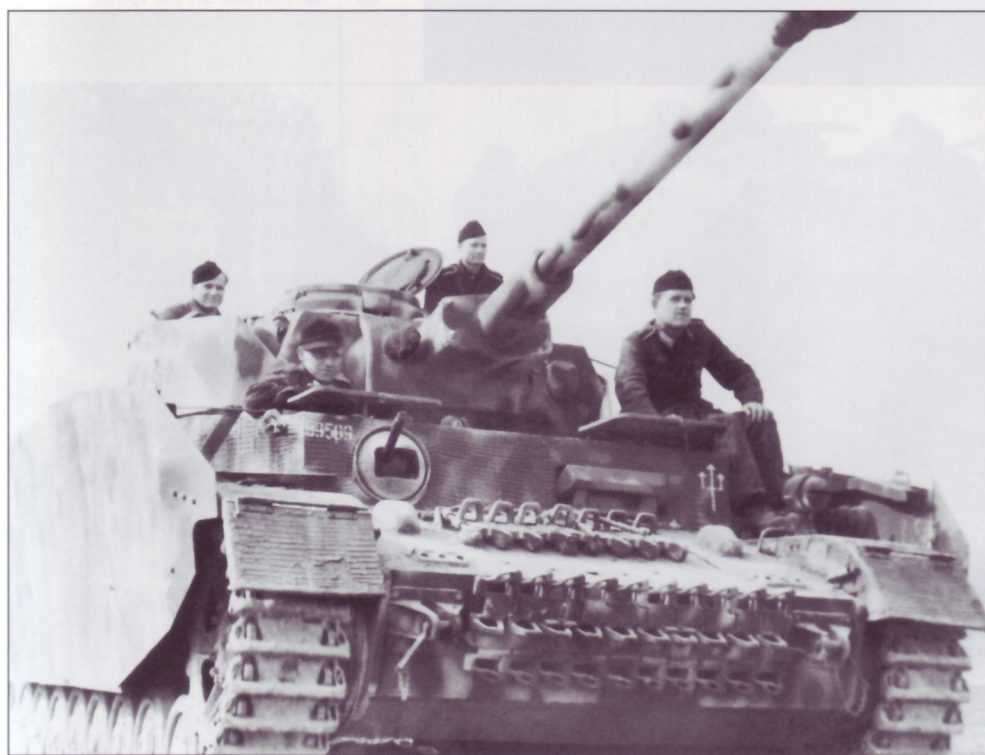
A pair of Pz.Kpfw.IV Ausf.Hs lead Tiger Is of SS-Division "Das Reich" along a forest track, on the Ostfront. The lead panzer is identified as an Ausf.H by the new drive sprocket which could not be fitted to an Ausf.G hull, unless the transmission and final drives were also changed. It has a single-piece lid on the commander's cupola as well as Zimmerit anti-magnetic mine paste, which was applied at the factory to panzers beginning in September of 1943. Note the cut-out portion of the small Schürzen plate just over the drive sprocket. The panzer is finished in the base of dunkelgelb RAL 7028 and has only a white-outlined, black balkenkreuz visible on the turret Schürzen. Other panzers in the column have the divisional insignia left-over from "Operation Zitadelle" (a horizontal bar with a pair of attached vertical bars, in white), which took place the previous July.
